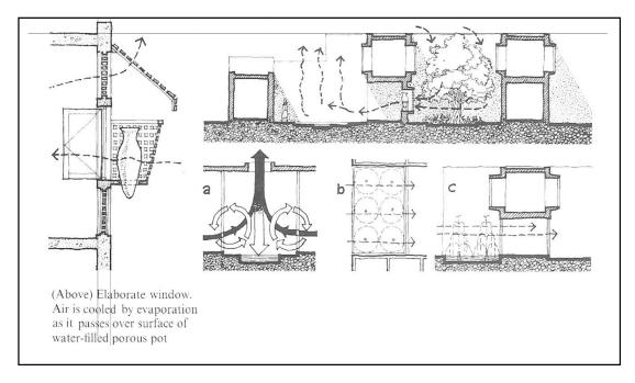
Figure 2. Evaporative coolers in front of window hoods in arid climate and wind convection over interior water pools. Source: Konya, A. Design Primer for Hot Climates, London: The Architectural Press Ltd. 1984.
