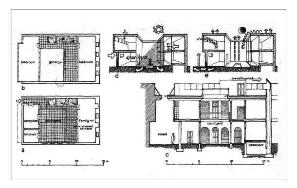
Figure 3. Enclosed Courtyards and Wind Towers as means of cooling the house interiors in arid regions. Source: Konya, A (1984) Design Primer for Hot Climates. London, The Architectural Press Ltd.
